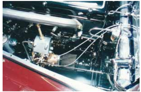
The Zenith updraft carburetor in the engine compartment.
