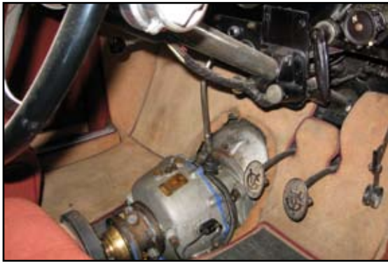
The Cotal Pre-Selector Gearbox exposed as it is repaired.
