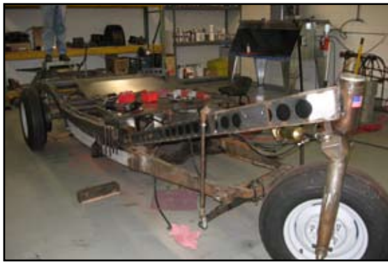
The chassis of the 1932 Dymaxion awaits paint & a new body!
