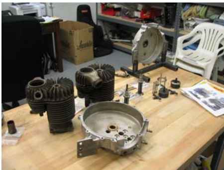
Above: 1917 Harley Davidson J engine that will power a replica Leyat Helica.
