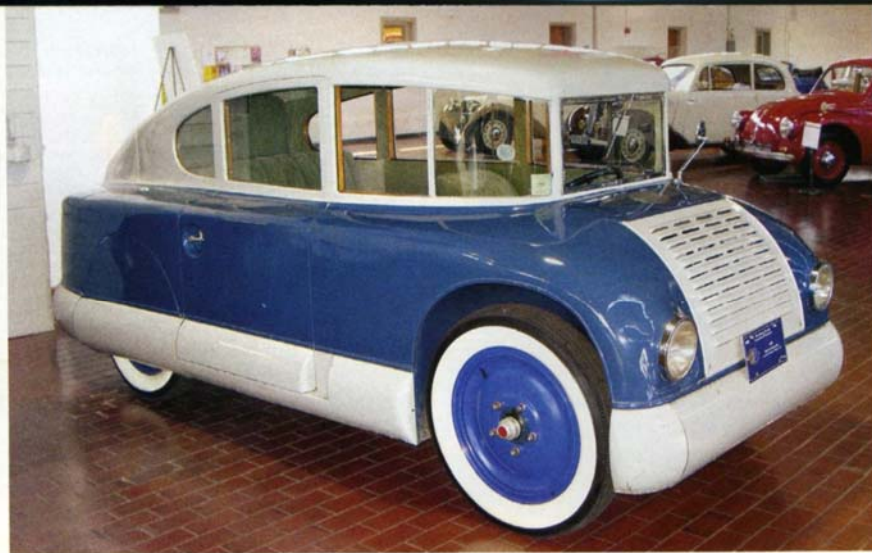
It's wild to learn that this aluminum-bodied, one-door Martin Aerodynamic Car was built in 1928 at a cost of $17,000; its airplane-type suspension doesn't use springs
